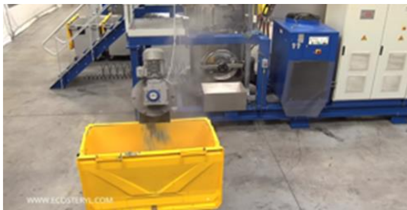
Fig. 7 Microwave sterilization process shredded (www.ecosterile.com)
