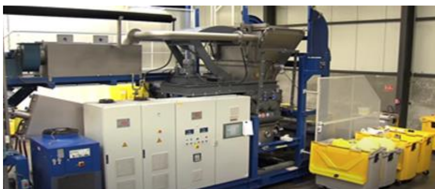
Fig. 6. Hazardous medical waste microwave treatment facility https://www.ecosteryl.com
